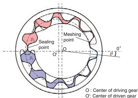
**Fig. 3** Pressure acting in internal gear pump
