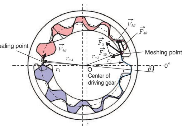
Fig. 7 Forces acting on driving gear
