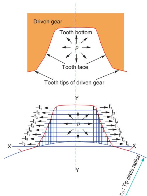
Fig. 5 Pressure and force acting on tooth
