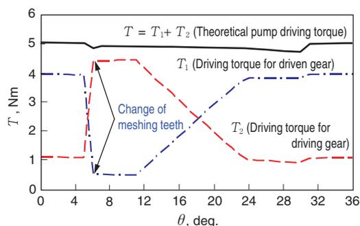
Fig. 11 Torques for driving each gear and pump driving torque
