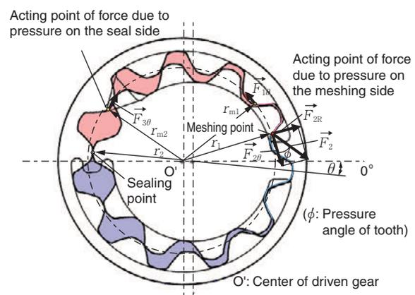
Fig. 6 Forces acting on driven gear
