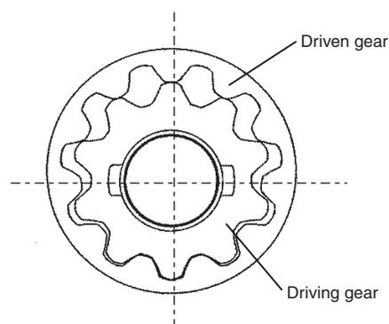
**Fig. 1** Configuration of internal gear pump without crescent
