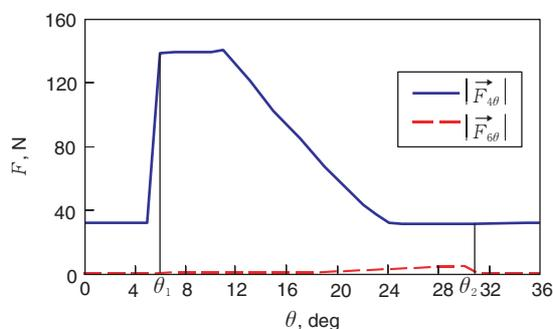
Fig. 10 Change of forces acting on driving gear
