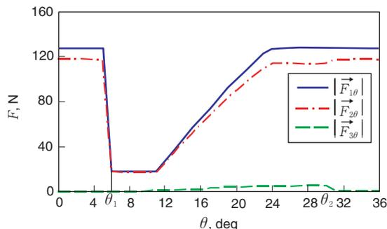
Fig. 9 Change of forces acting on driven gear
