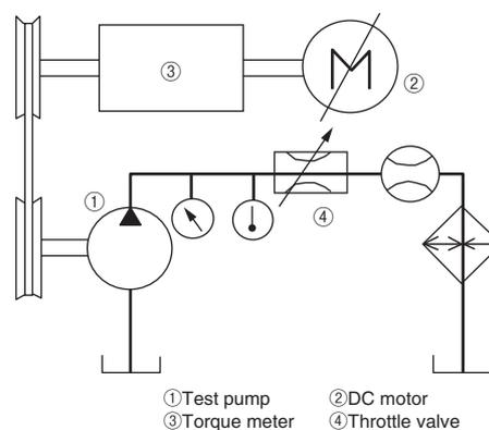
Fig. 13 Test circuit
