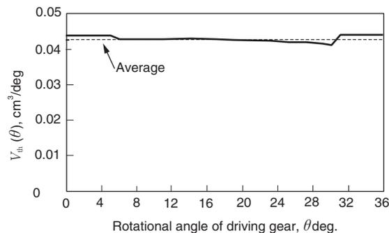
Fig. 12 Change of pump displacement per degree
