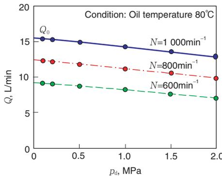
Fig. 14 Real flow of pump
