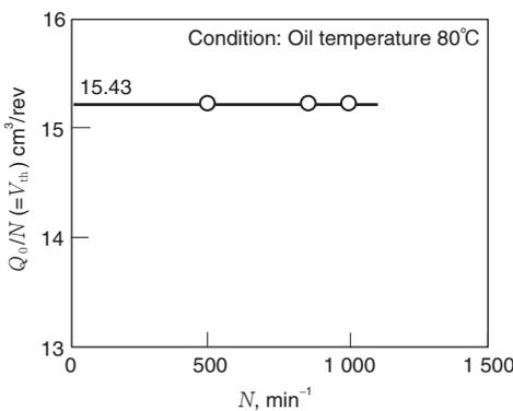
Fig. 15  $V_{th}$  estimated from measured flow
