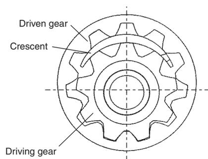
**Fig. 2** Configuration of internal gear pump with crescent
