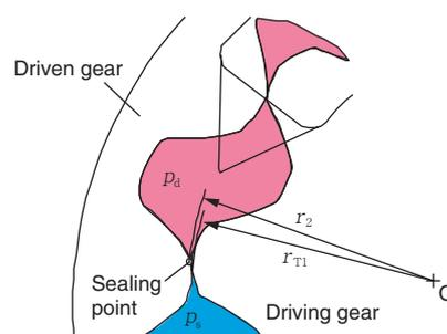
**Fig. 4** Tip circle radius and seal radius of driven gear
