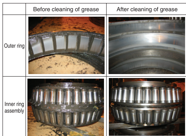
Fig. 8 Post-use appearances of bearing with high-sealing performance seal
