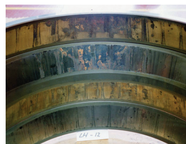
Fig. 4 Example of work roll neck bearing failure
