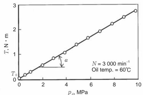
Fig. 2 Relationship between oil pump pressure and torque
