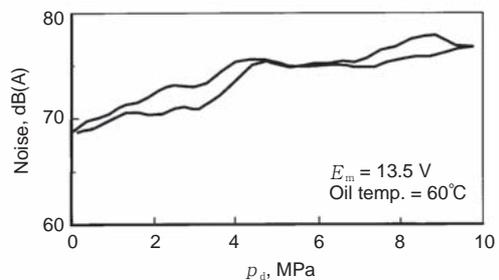
Fig. 12 Noise characteristic of electric motor-driven oil pump
