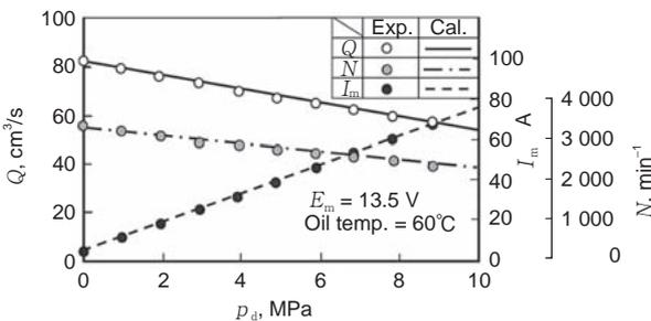
Fig. 9 Flow rate, electric current and motor speed in relation to delivery pressure
