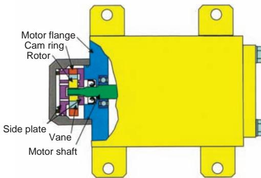
Fig. 1 Structure of electric motor-driven oil pump
