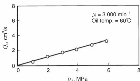
**Fig. 3** Characteristic of leakage flow in oil pump
