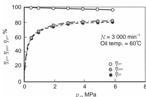
**Fig. 5** Efficiencies of oil pump
