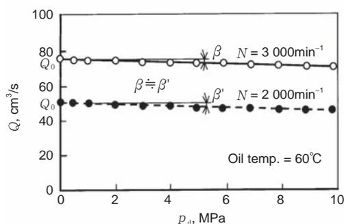
**Fig. 4** Relationship between oil pump pressure and flow rate
