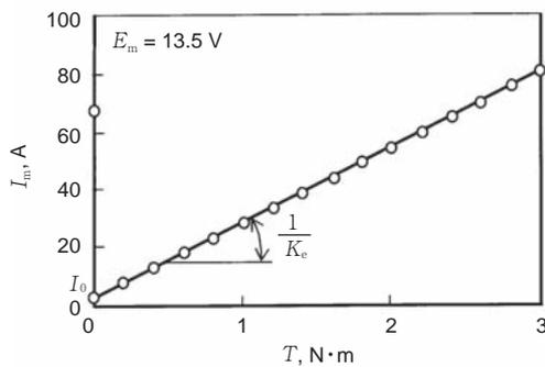
**Fig. 8** Relationship between electric motor torque and current
