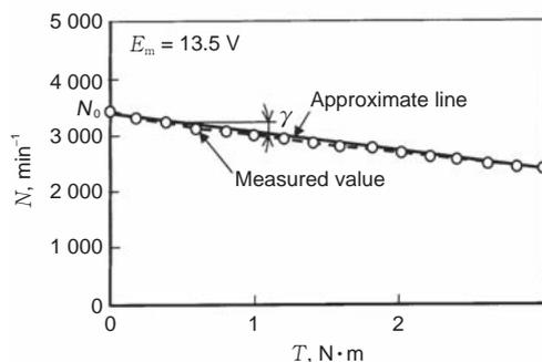
**Fig. 6** Relationship between electric motor torque and motor speed
