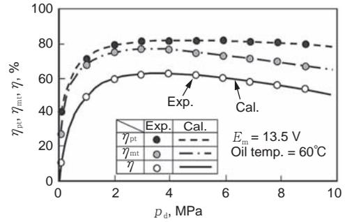
Fig. 10 Efficiencies of electric motor-driven oil pump
