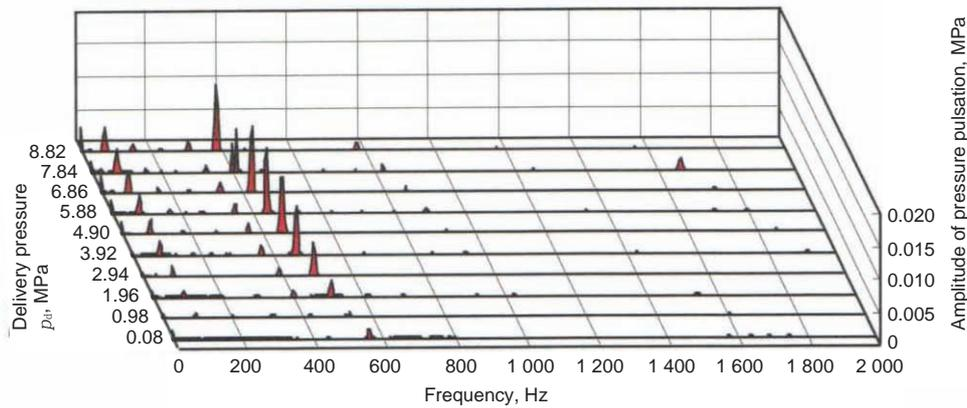
**Fig. 11** Pressure pulsations of electric motor-driven oil pump
