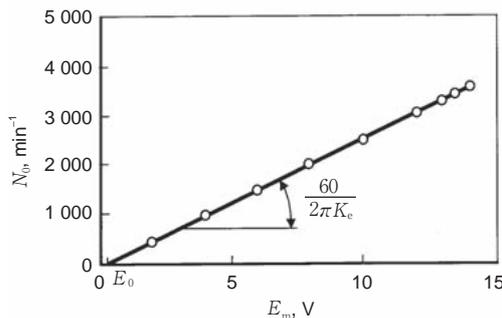
**Fig. 7** Relationship between electric motor input voltage and motor speed
