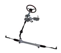
For FR sports cars, JTEKT has developed a column type electric power steering system with improved steering feeling. The features of this newly developed steering system are introduced below.
