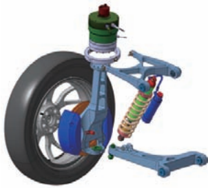
Fig. 7 Wheel individual steerable front axle of the research vehicle SpeedE
