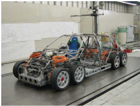
Fig. 5 Integrated platform with upper frame
