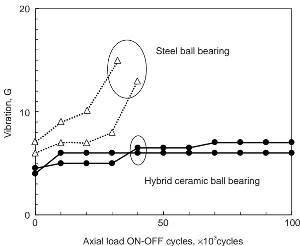
**Fig. 17** Durability test results in 20 000km used oil
