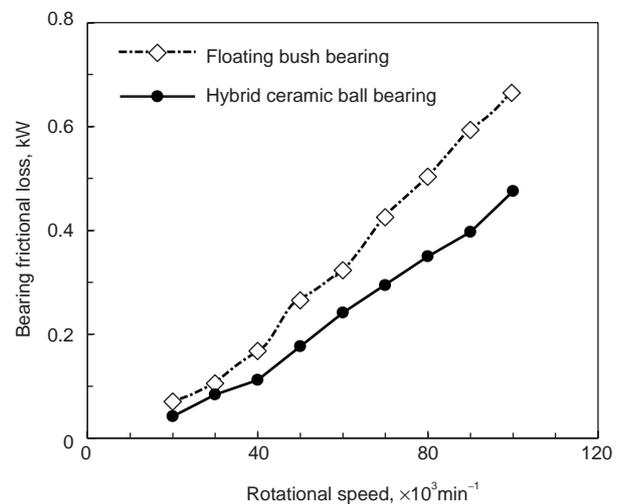
**Fig. 13** Bearing frictional losses during acceleration v.s. rotational speed
