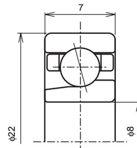
Fig. 2 708 test bearings dimensions
