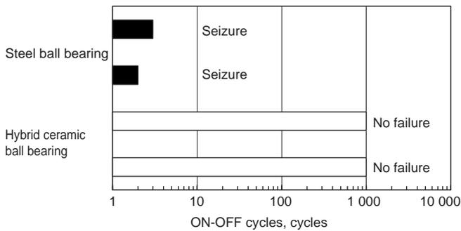
**Fig. 22** Repeated Go-Stop rotational speed durability test
