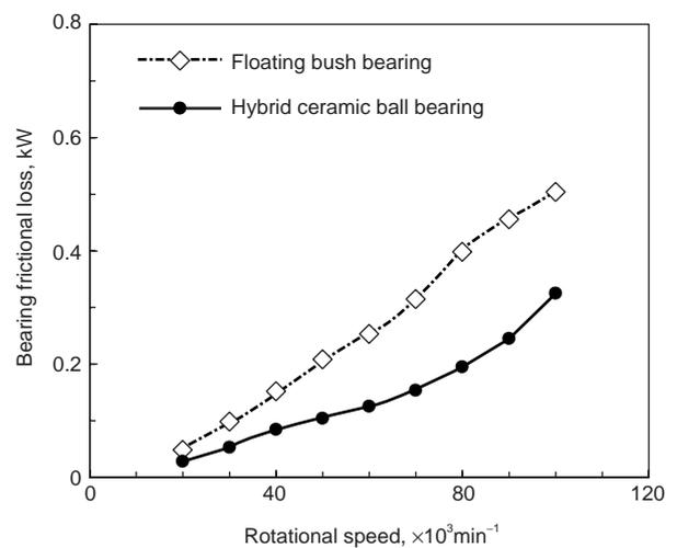
**Fig. 14** Bearing frictional losses during deceleration v.s. rotational speed
