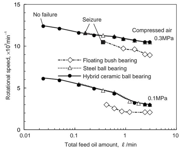
**Fig. 9** Relationship between rotational speed and total feed oil amount
