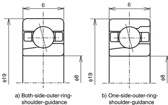
Fig.6 798 test bearing dimensions
