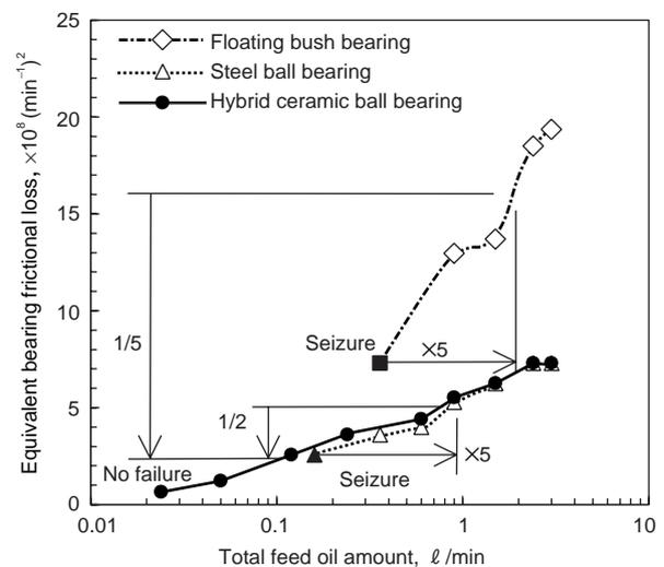
**Fig. 10** Equivalent bearing frictional loss v.s. total feed oil amount
