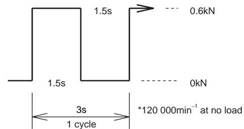
Fig. 15 Cycle of axial loading
