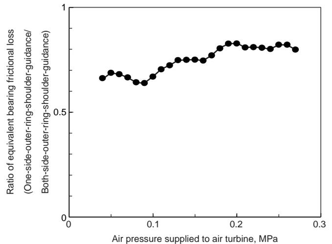
Fig. 7 Equivalent bearing frictional loss v.s. compressed air pressure (Influence of cage guidance)
