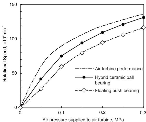
**Fig. 3** Relationship between rotational speed and compressed air pressure
