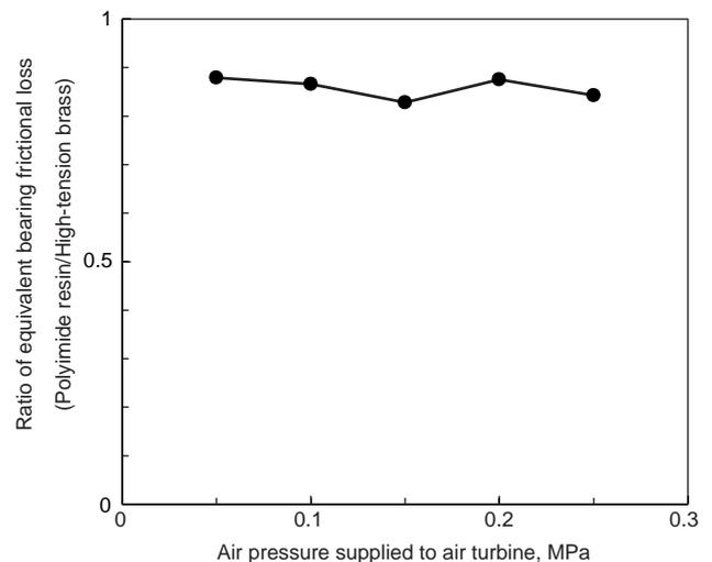
**Fig. 5** Equivalent bearing frictional loss v.s. compressed air pressure (Influence of cage materials)
