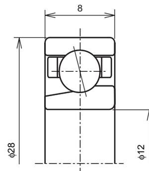
Fig. 8 7001 test bearing dimensions
