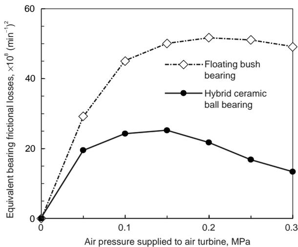
**Fig. 4** Equivalent bearing frictional loss v.s. compressed air pressure
