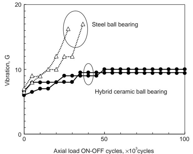
**Fig. 18** Durability test results in contaminated oil with 0.027mm high-speed steel powder
