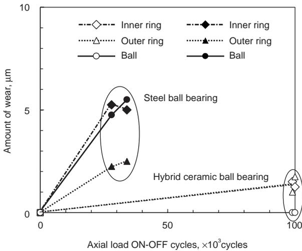
**Fig. 19** Component wear in contaminated oil with 0.027mm high-speed steel powder
