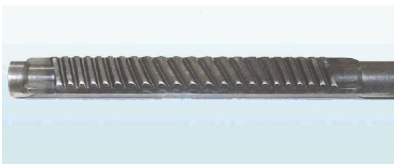
Fig. 5 Variable gear-ratio rack bar
