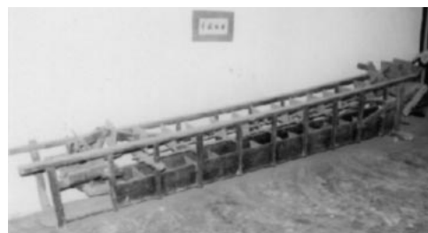
Fig. 1 A whole picture of dragon-bone water lift 3)
