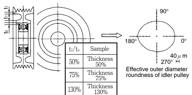
Fig. 15 Shape of developed idler pulley (without reinforcement ribs)
