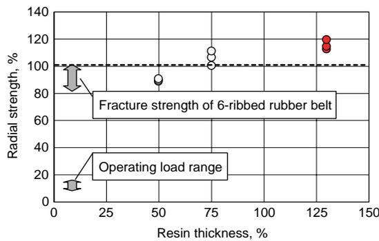
Fig. 19 Measurement result of radial strength
