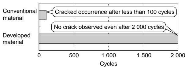
Fig. 13 Result of thermal shock test
