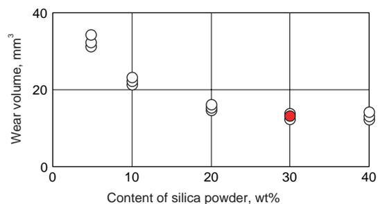
Fig. 6 Relation between amount of silica powder and wear
