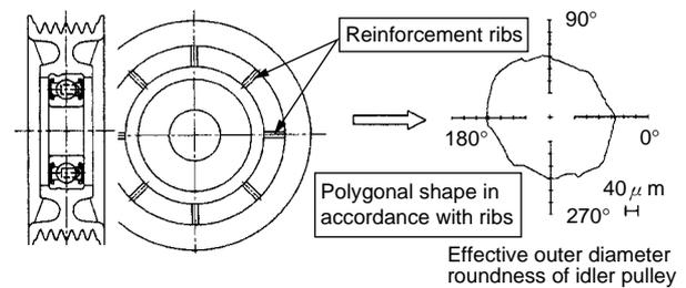
Fig. 14 Shape of conventional idler pulley (with reinforcement ribs)
