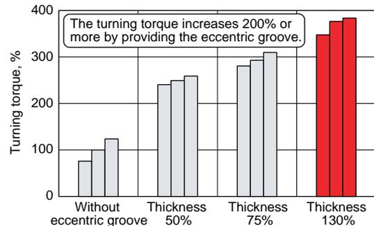
Fig. 20 Measurement result of turning torque
