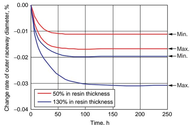
Fig. 21 Change rate of outer raceway diameter
