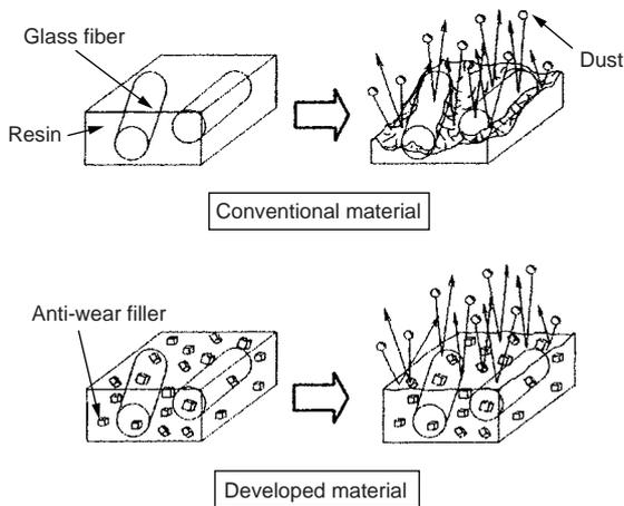
Fig. 3 Mechanism of wear progressing
