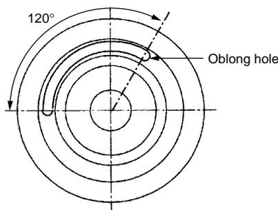
Fig. 23 Sample configuration for fatigue test
