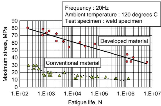
Fig. 12 Result of fatigue test at high temperature
