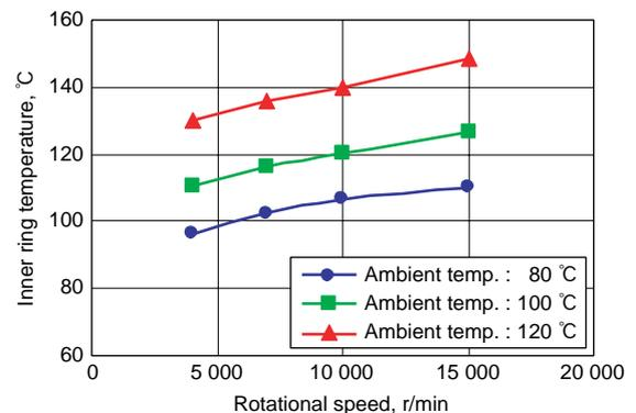
Fig. 25 Measurement result of inner ring temperature
