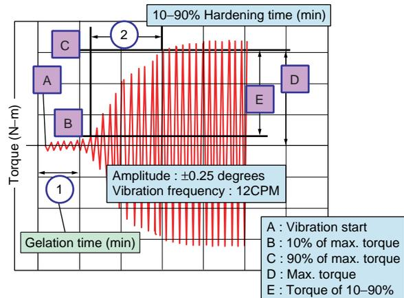
Fig. 10 Measurement result of hardening characteristics
