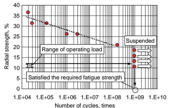
Fig. 24 Result of rotational fatigue test
