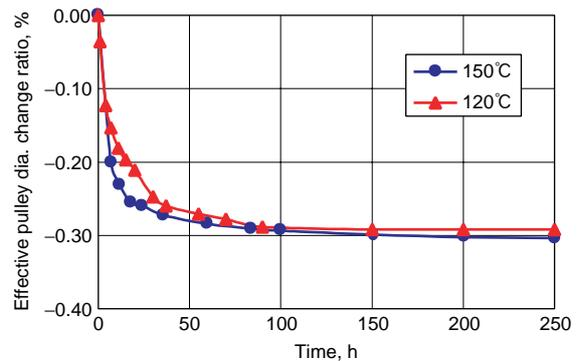
Fig. 16 Measurement result of change rate in effective pulley diameter.
