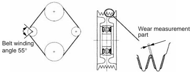
Fig. 7 Belt layout and wear measuring section
