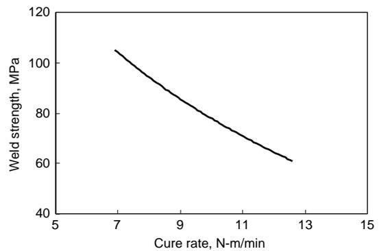
Fig. 11 Relation between cure rate and weld strength
