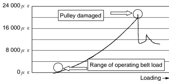
Fig. 18 Measurement result of strain at the damaged area
