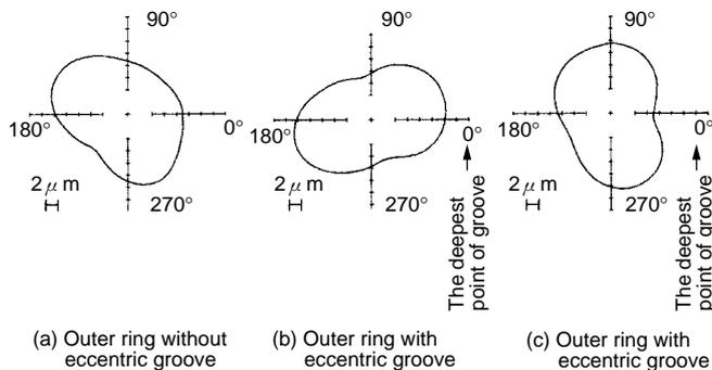
Fig. 22 Roundness of outer ring (130% resin thickness)
