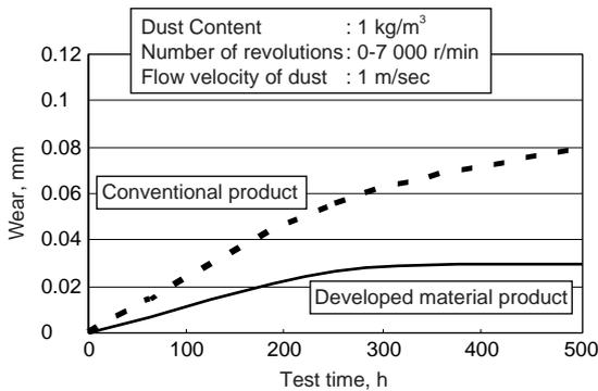
Fig. 8 Result of dust durability test
