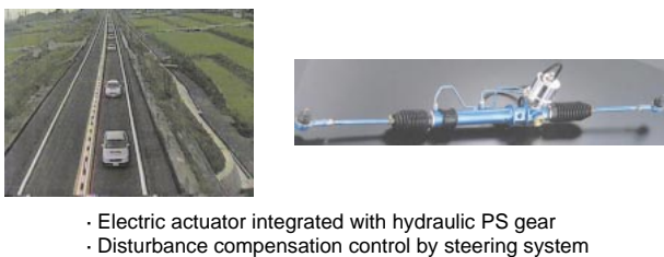
Fig. 9 Disturbance compensation control in automatic steering control system
