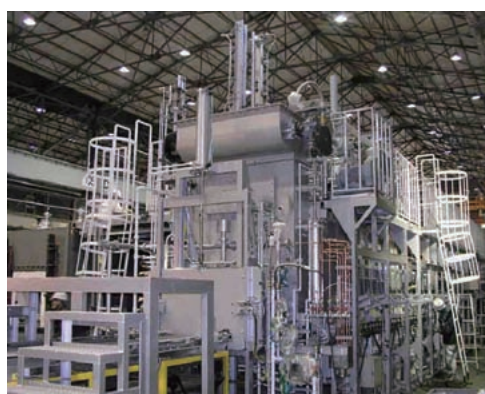
図1 省エネルギータイプ高性能連続ガス浸炭炉の外観 Appearance of energy-savings-type-high-performance continuous carburizing furnace
