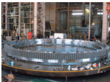
図22 軸受外観 Appearance of bearings
