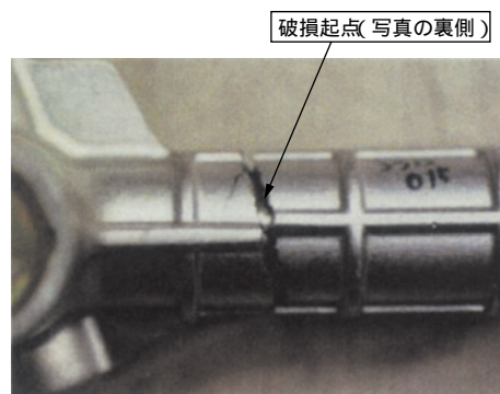
図7 逆入力静的強度試験の破損部 Fracture point during static reverse input strength test
